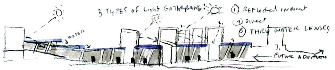
Holl’s early conceptual drawing of an elevation (above) sketches out the flow of natural light through the exterior. In an exploded axonometric (below), the aboveground “lenses” and submerged galleries are represented as distinct layers.
